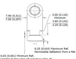
(applies to top edge of gasket or edge of crimp, whichever is higher)
