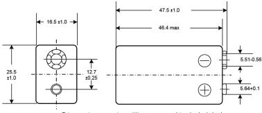
Dimensions are in millimeters and include label.
