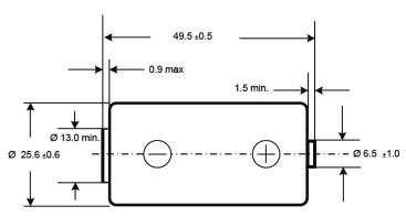
Dimensions are in millimeters and include label.
